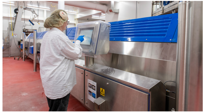
Rhino Foods can preset the wave frequency, speed of the conveyor belt, and other process parameters for rapid change-outs between products. Messer's versatile Wave Freezer is also modular; freezer tunnel sections can be added as production needs grow.
