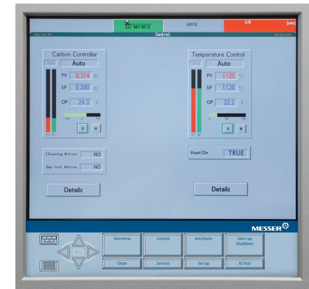
User-friendly customer interface for real-time monitoring and dynamic adjustment of furnace atmosphere
