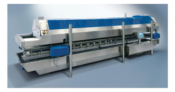
The Messer Wave Freezer is a multi-purpose freezer which can efficiently freeze individually quick-frozen (IQF) as well as trayed products. The flexible and versatile technology, which employs cryogenic medium, combines a standard tunnel with a mechanical system that agitates the product as it is conveyed through the freezer. Thus, the freezer has the ability to crust freeze products individually, irrespective of shape, form and orientation, and without affecting the integrity of the product.
