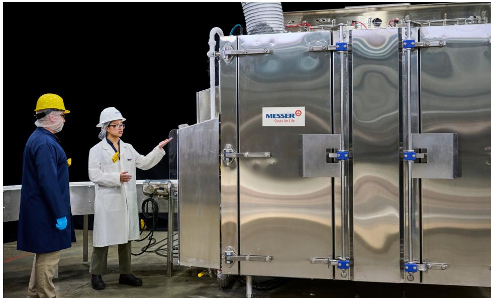
*Messer's spiral freezers deliver 750 to 15,000 lb/hr of throughput in a compact footprint—ideal for boosting existing freezing capacity or handling full freezing applications.*
